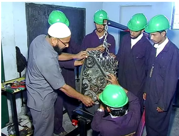
Students are shown how to install Engine belt
